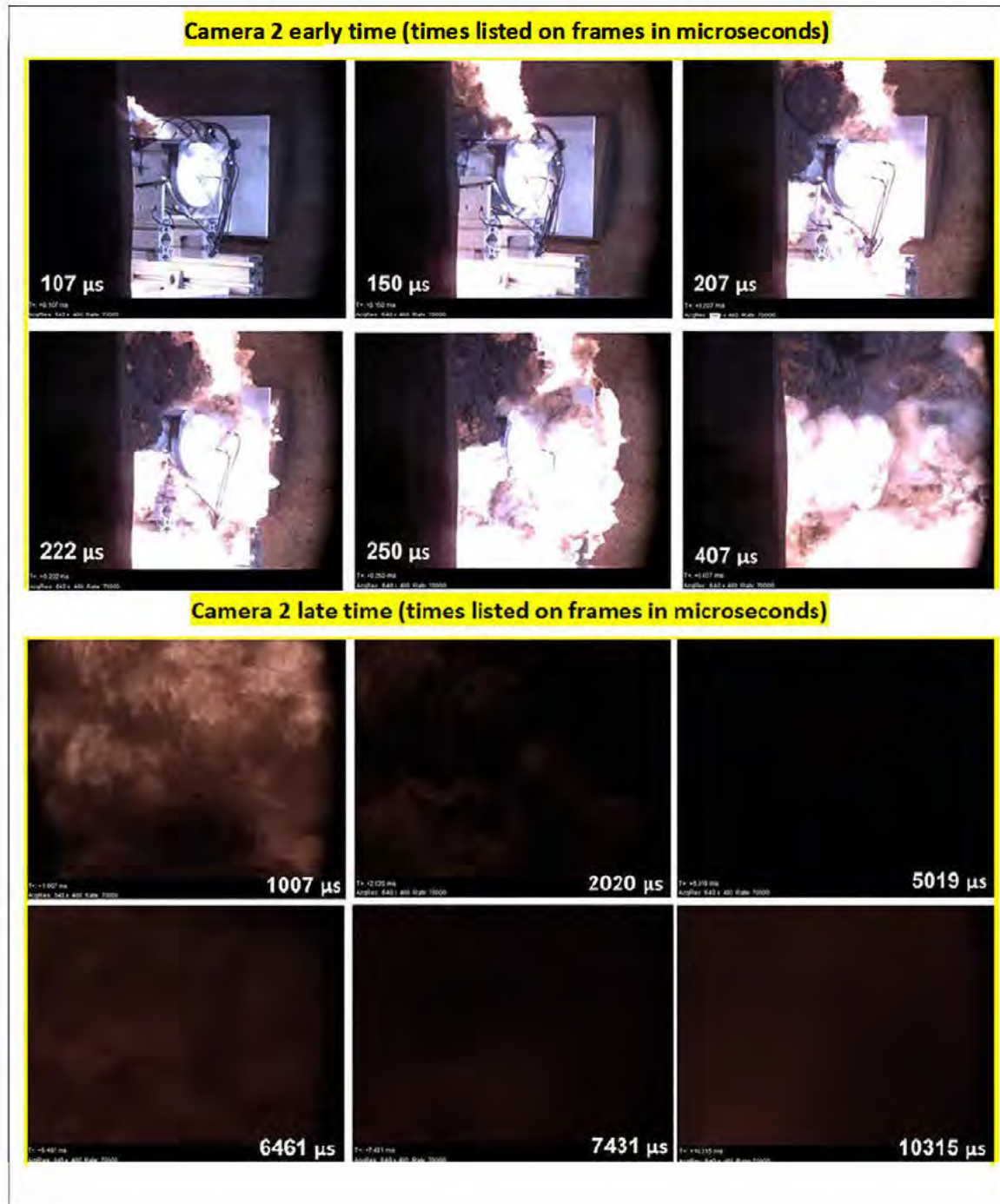
Figure B25. Still images from camera 2 (45° off tank centerline) high-speed imaging. Top: Early time detonation products moving angled towards the camera. Note that there was no discernable plastic dust cloud, or the aluminum end cap projected into the adjacent catcher tank. The early time is front lighted with
