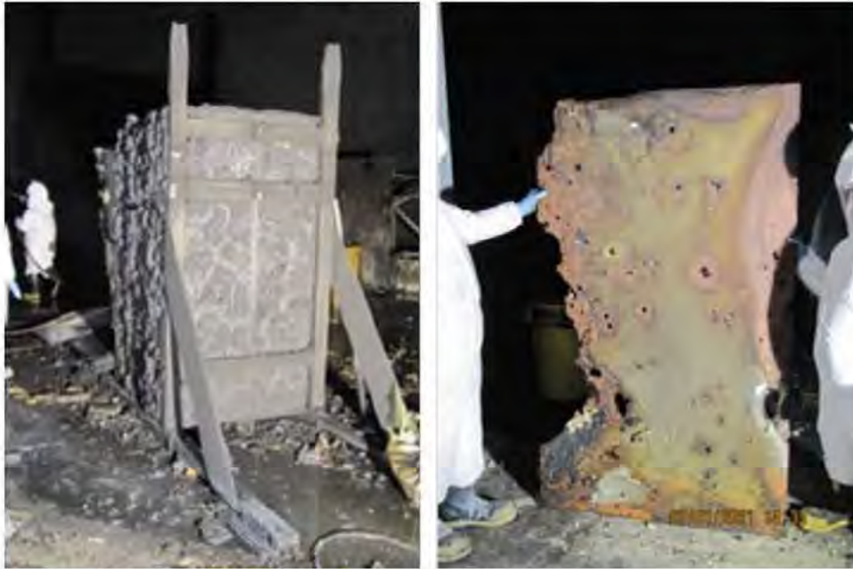
Figure A5: Post-shot images showing charred frag catcher foam and aluminum stand.
