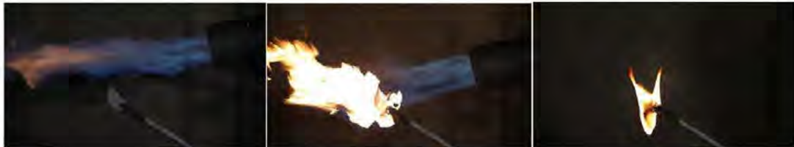
Figure B7: 3D-printed ABS in flame test. Left: prior to exposing the sample to direct flame. Middle: holding flame on sample (note that change in flame color and intensity indicates combustion other than propane). Right: 3D-printed ABS burning to completion after the flame was removed.
