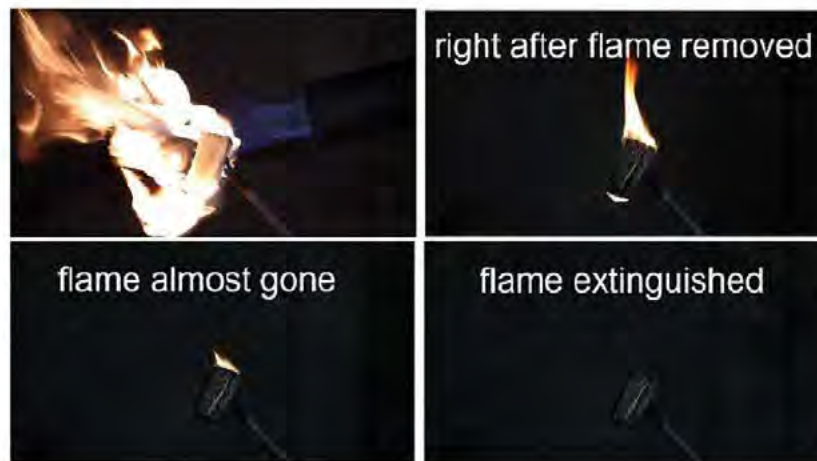
Figure B10: Flame exposure test on FR-3703 where the flame is removed after ignition. Upper Left: torch igniting the FR-3703 foam (note the change in flame color and intensity indicating combustion other than propane). Upper right: Flame removed, sample continues to burn, but quickly diminishes in surface burning. Lower Left: Flame quickly extinguishes. Lower right: From the time the torch was removed to the time no flame was visible ranged from ~15-25 seconds.
