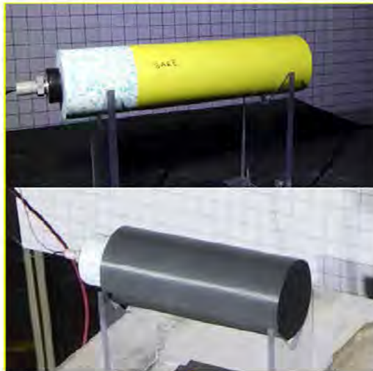
Figure B4: Top: Experimental setup for detonation shock-pulverization of ABS experiment and the control experiment. Bottom: Images of actual setups for control and shock pulverization experiment.
