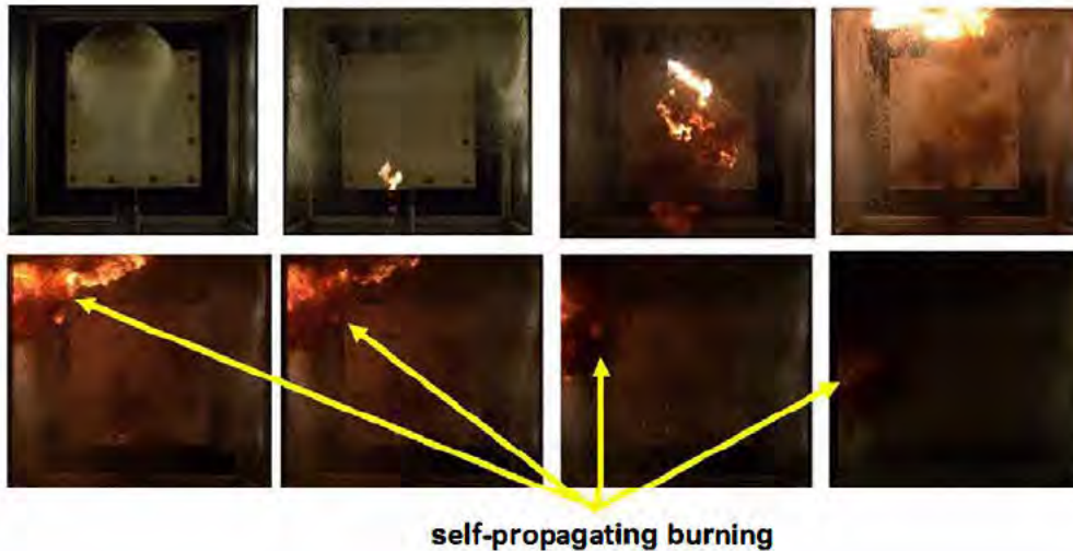
Figure B17: Images taken from the DFIC experiments on FR-3703 foam. The initial two images (upper left images) were artificially brightened to illustrate the powder cloud being dispersed. Some self-propagating reaction was observed. The squib was fully consumed shortly after the upper right-most image, the remaining bottom four images are all thought to be self-propagating combustion reaction.
