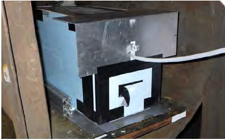
Figure B23. Ridged polystyrene foam box used to insulate the Icepick assembly while being cooled to -54\text{ }^{\circ}\text{C} . The center of the 3D-printed ABS billet was monitored with a thermocouple. The entire charge was cooled to -64\text{ }^{\circ}\text{C} , then the insulation was removed, and the tank closed. The shot occurred when the 3D-printed ABS thermocouple read -53\text{ }^{\circ}\text{C} .
