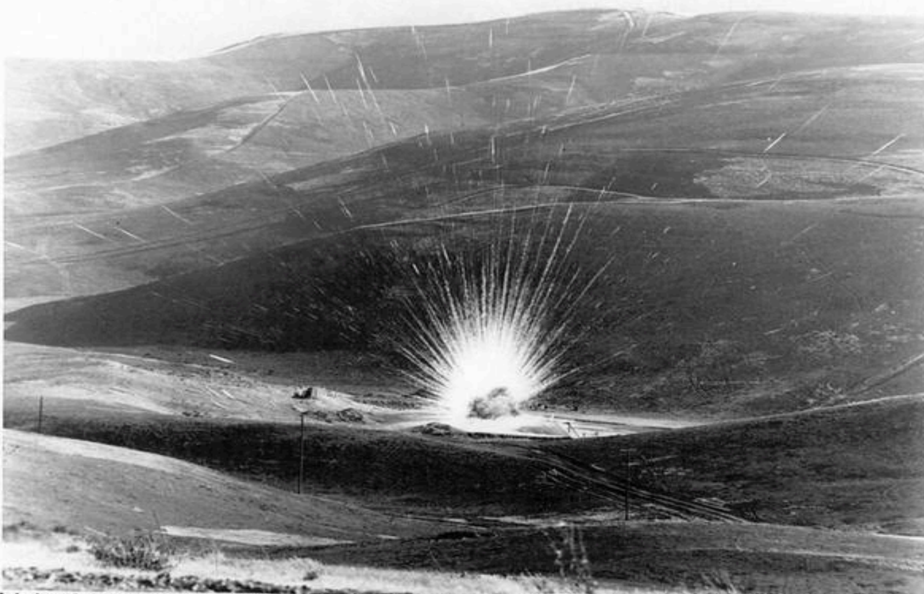
Hydrodynamic (bomb core) test on a firing table at Site 300, 1961. The bright "streaking" effect in the photo is likely from shards of pyrophoric metal, such as Uranium 238, hurtling through the air. U-238 is one of the contaminants of concern in the Site 300 Superfund cleanup. Photo: LLNL
