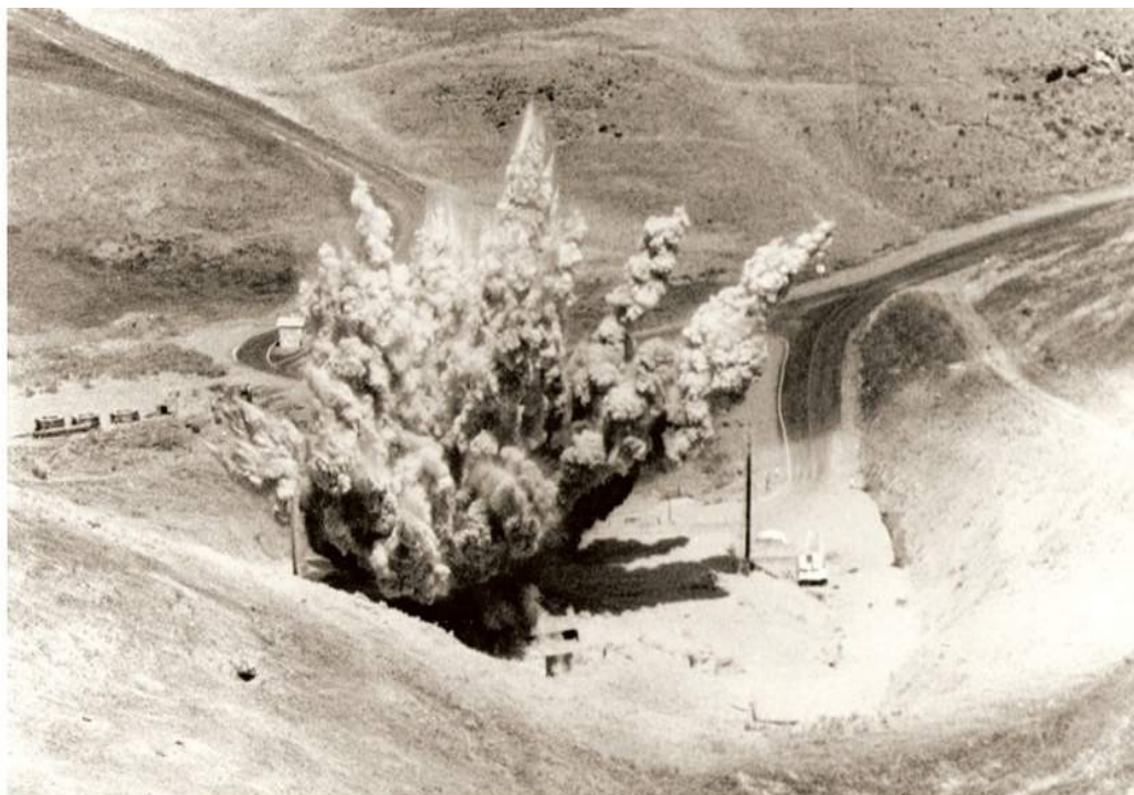
Hydrodynamic (bomb core) test on firing table at Site 300, 1984. Note size of building on left in comparison to blast. These tests are ongoing at Site 300. Debris from these tests are among the contaminants that need to be remediated under the Superfund cleanup. Photo: LLNL
